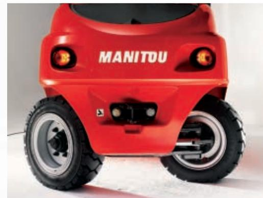
In aisles, its compactness and **very tight turning circle due to a steering axle with built-in cylinder provides incredible manoeuvrability.**
