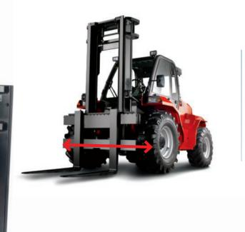
Its **width** ensures the fork-lift truck has better stability for extra safety for lateral loading.
