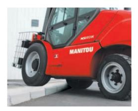
The low-pressure tyres absorb the shock of driving over obstacles and give perfect grip on slippery surfaces. In addition, the front axle is fitted with a differential lock as standard.
