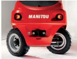
In aisles, its compactness and very tight turning circle due to a steering axle with built-in cylinder provides incredible manoeuvrability.
